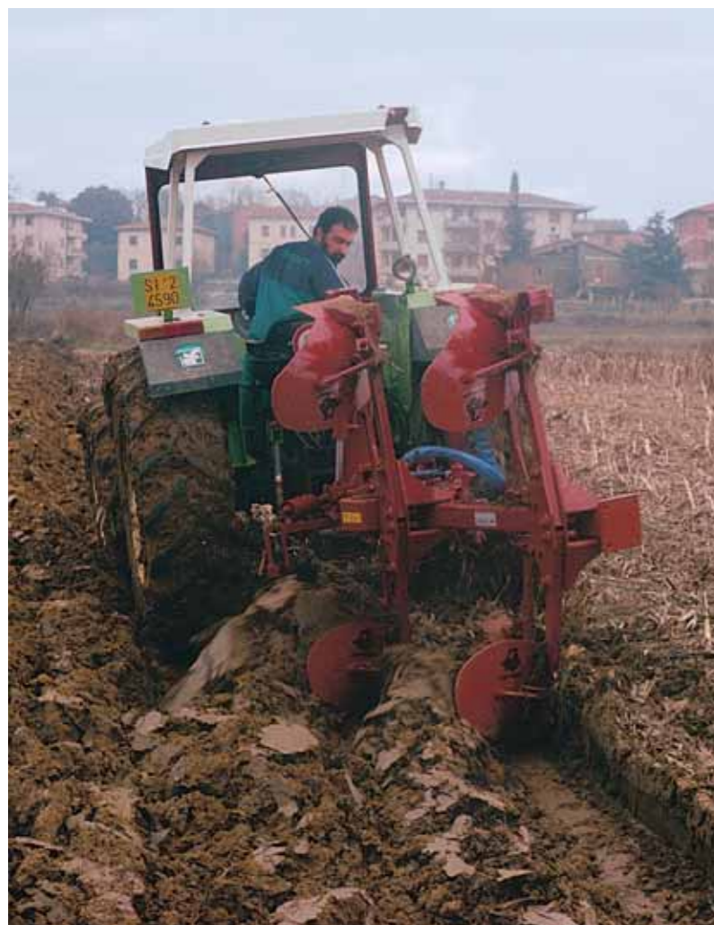
Mod. D/VQ ARATRO QUADRIVOMERE REVERSIBILE Reversible four furrow plough Charrue reversible quadrisoc Arado reversible quadrisurco
